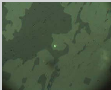
100x magnification image of a specimen of lapis lazuli. Lazurite mineral is seen in the image as the darker shaded regions.
